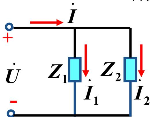
$$\begin{aligned} Z &= \frac{Z_1 \cdot Z_2}{Z_1 + Z_2} = \frac{5 \angle 53^\circ \times 10 \angle -37^\circ}{3 + j4 + 8 - j6} \Omega \\ &= \frac{50 \angle 16^\circ}{11.8 \angle -10.5^\circ} \Omega = 4.47 \angle 26.5^\circ \Omega \end{aligned}$$
